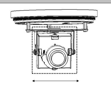
Module can be adjusted up and down
